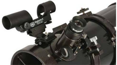
For larger tubes, insert the intermediate adapter ④ between tube and adapter ③ (as shown in the image).
