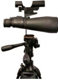
If your binoculars are attached via a photo screw on the front of the middle bridge and an angular or L-adapter on a tripod, attach the SkySurfer III on the adapter. Run the fastening screw of the tripod adapter through the hole of SkySurfer adapter and screw both on your binoculars. So you can use the SkySurfer also with large binoculars with a small field of view. On binocu-
