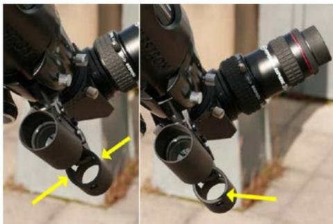
the rear barrel. On the right is the sight when the sun is not centered and the shadow only cuts the rear ring (yellow arrow). You may need to re-adjust the viewfinder for solar observation, or mark the intersections of the shadow on the rear section. Please follow the safety instructions of your telescope when you observe the Sun. You can find safe solar filters on <http://astrosolar.com>.
